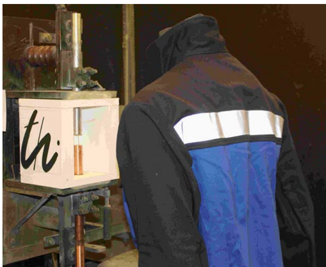
Fig. A 2-1 Test setup, Box test method
