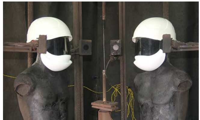
Fig. A 2-2 ATPV Test setup
